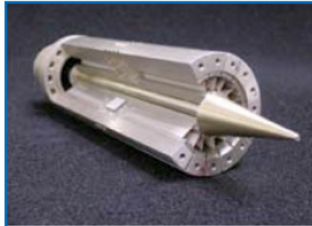
Figure 5: Physical implementation of spatial combining coaxial architecture in Spatium amplifier
